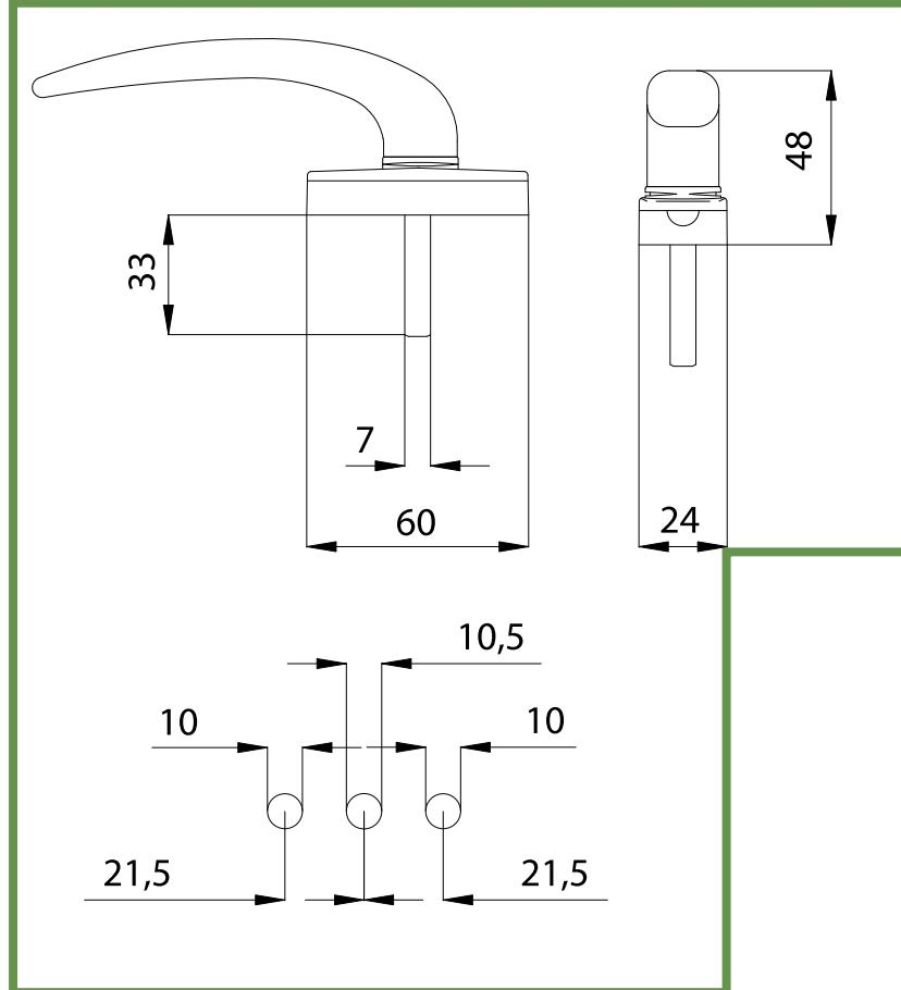
Hand handle for use on mechanisms which move the rods that allow closure of the windows. Equipped with a nylon mechanism for the positioning of the handle at 90° and 180°.
