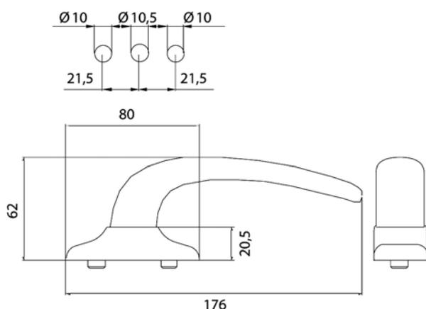
Right- or left-hand handle for use on mechanisms which move the rods that allow closure of the windows. Equipped with a ball mechanism for the positioning of the handle at 90° and 180°.
